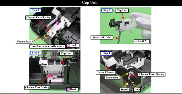
When installing the Cap Unit, follow the instruction below.
