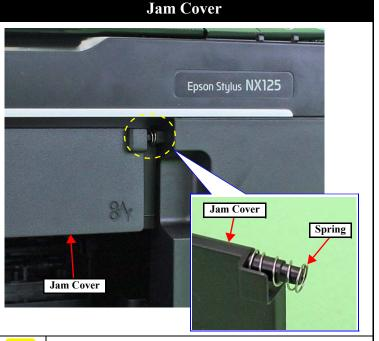
When removing the Jam Cover, be careful not to lose the spring installed to the dowel on the right side.
