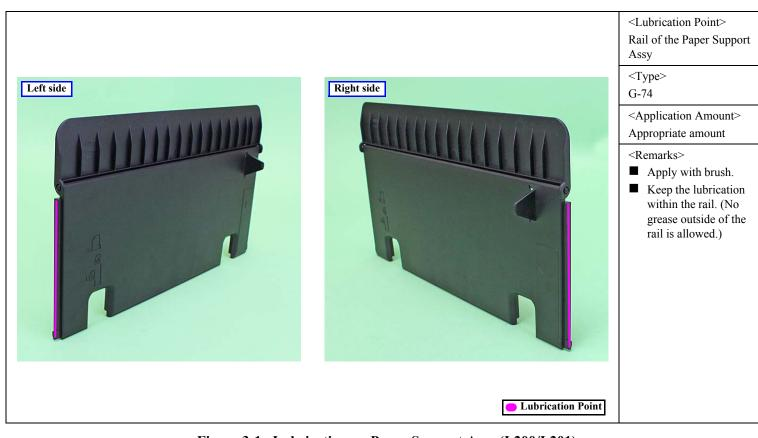
Figure 3-1. Lubrication on Paper Support Assy (L200/L201)
