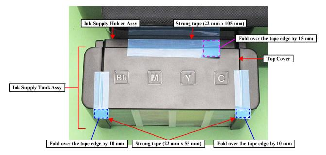
Figure 1-5. Securing the Ink Supply Tank Assy
