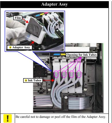
When installing the ink tubes to the Adapter Assy, insert the ink
