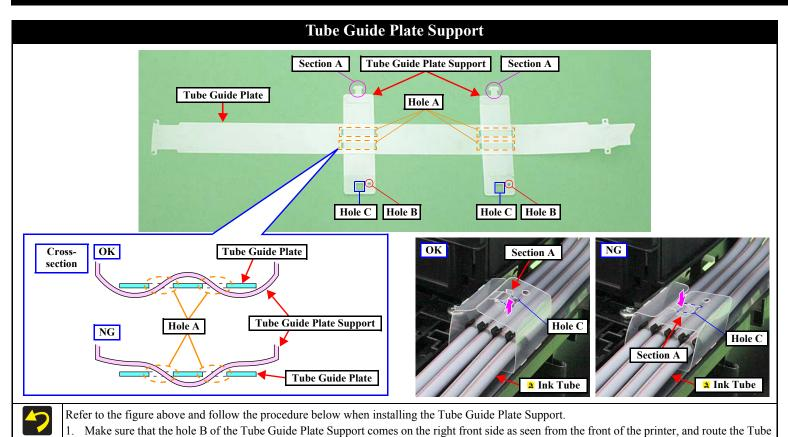
Insert the section A of the Tube Guide Plate Support into the hole C of the Tube Guide Plate Support up from the bottom as shown in the "OK"
