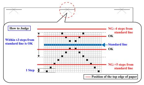
Figure 2-1. Top Margin Adjustment Printout Pattern
