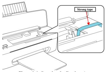
Figure 1-4. Securing the Carriage Assy
