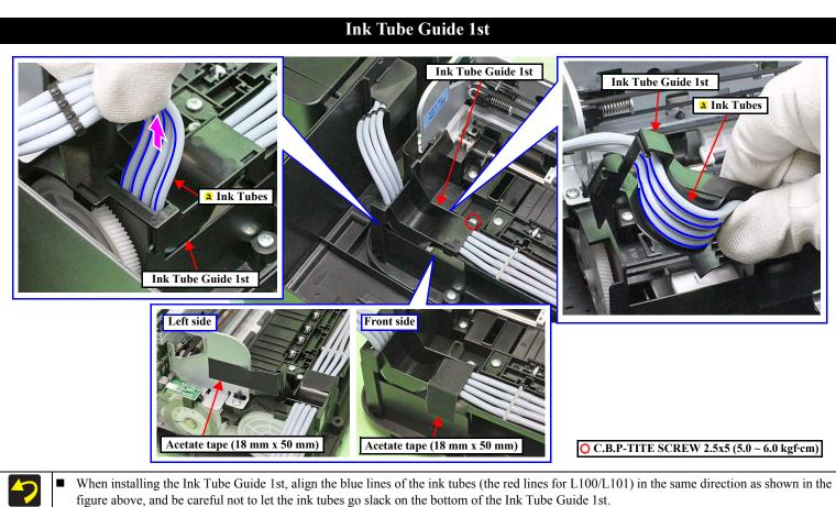
■ After securing the Ink Tube Guide 1st, pull the ink tubes from the Ink Supply Tank Assy side to make sure that the ink tubes are not caught.
