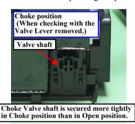
Figure 1-2. Opening/closing the Choke Valve
