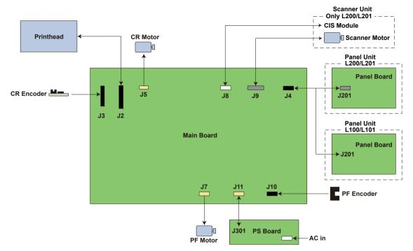
Figure 4-1. Connector Diagram
