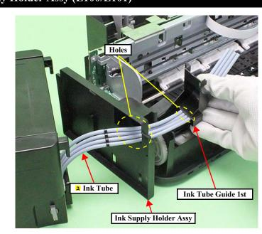
Follow the procedure below when removing the Ink Supply Holder Assy / Ink Tube Guide 1st. Remove the Upper Housing Assy. (p 30)
