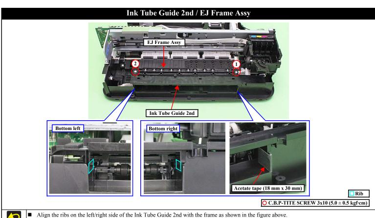
■ Tighten the screws of the Ink Tube Guide 2nd together with the EJ Frame Assy in the order indicated in the figure above.
