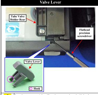
In order to prevent ink spill, make sure to close the Valve Lever
