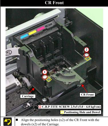
■ Tighten the screws in the order indicated in the figure above.
