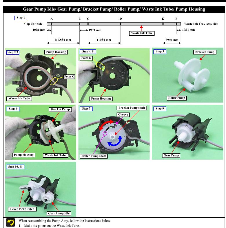
Insert the Waste Ink Tube in the hole of the Pump Housing with the red line of the tube set as shown in the figure above.
