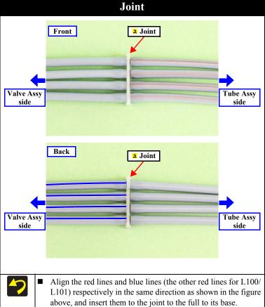
■ Be careful not to damage the ink tubes and joint.
