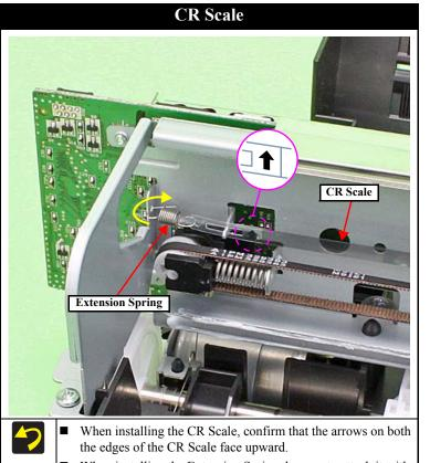
■ When installing the Extension Spring, be sure to attach it with its leg facing the rear of the printer.
