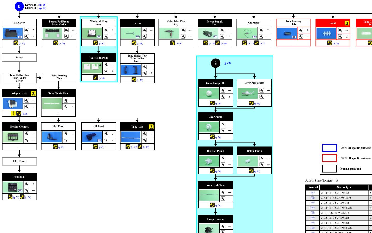
Flowchart 1-4. Disassembling Flowchart of Printer Mechanism Part (2)
