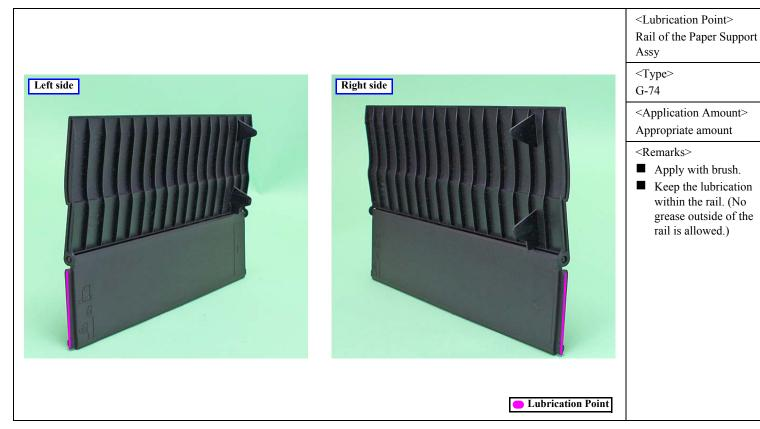
Figure 3-9. Lubrication on Paper Support Assy (L100/L101)
