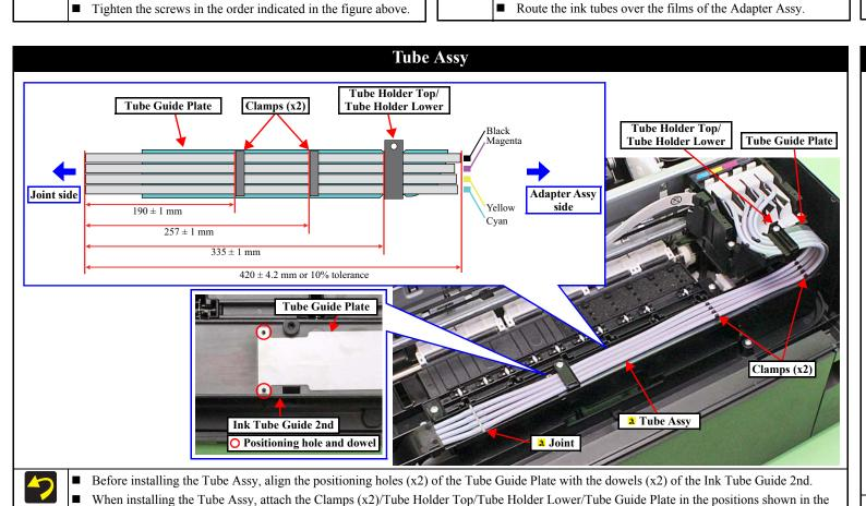
When installing the Tube Assy, align the red lines of the ink tubes in the same direction as shown in the figure above, and attach them without
